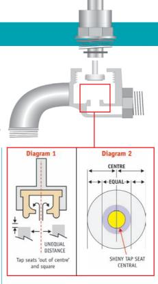
If this new shiny circle is complete and in the centre, (use a flashlight if difficult to see) then fit your new DoustValve™ complete with the bonnet and spindle. New body washers are supplied in the DoustGrease™ pack and they should also be fitted. The water entry inlet
